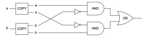
The above circuit still contains two crossed wires, which corresponds to swapping bits. We can make this explicit with a  $SW\!AP$  gate:
