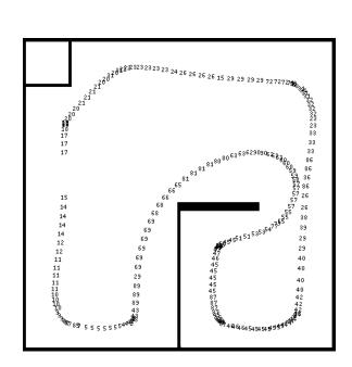
Figure 5: The path of the robot under control of the governor-trained network, showing the perceptual categories associated with each position as the robot moves clockwise around the environment.
